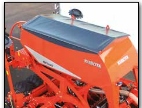
A close fitting hopper cover protects the seed from dust and water.
