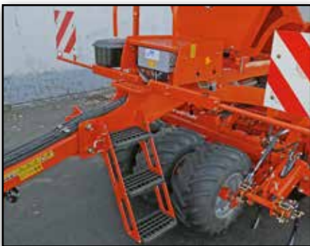
The loading steps and platform provide safe access for filling and inspection of the hopper.
