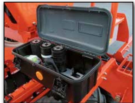
Calibration bag and scale is ready to hand and stored with the rotors well protected against dust in the toolbox.
