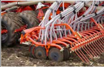
Double entry seed outlet: fertiliser application in the row
