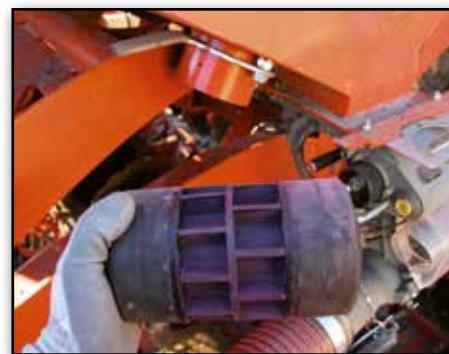
The metering device is easily accessible. To exchange rotors no tool is needed.
